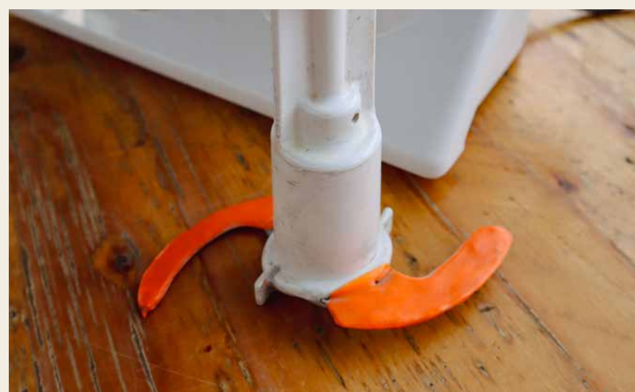
Food processor with Plasti Dip-coated blades used to extract wet seeds
