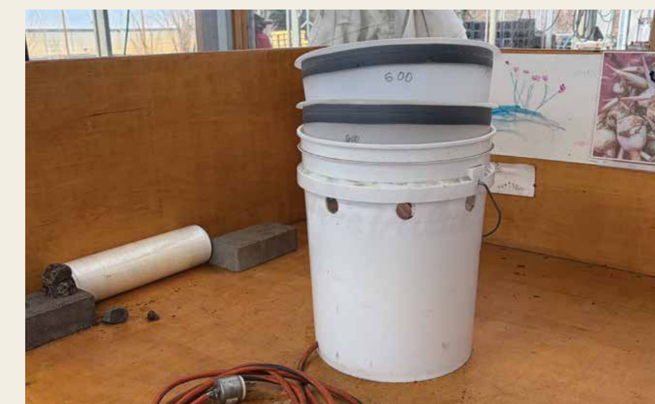
Seed dryer made from a five gallon bucket and fan
