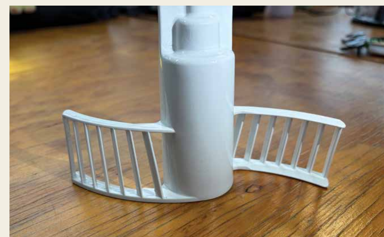
Food processor whisk attachment used to thresh dry seeds
