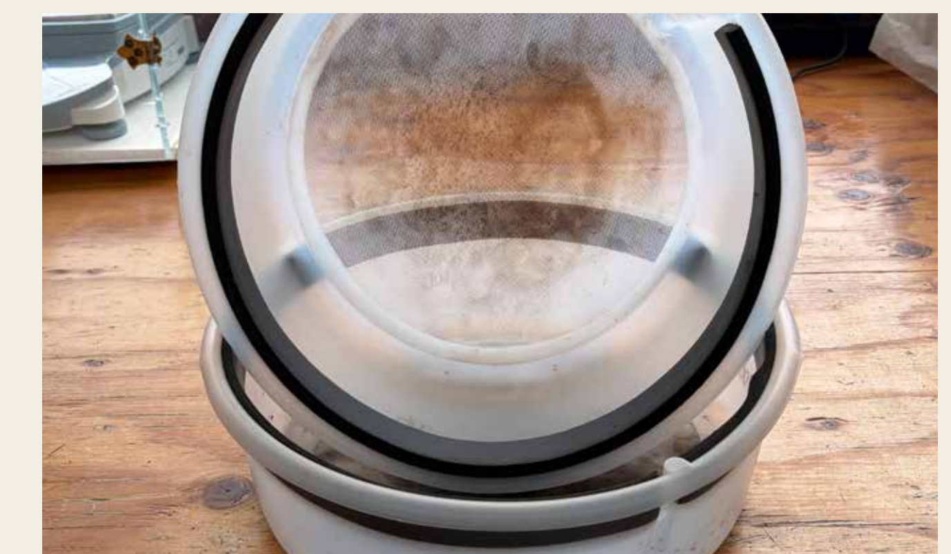
Dryer trays made from strainer inserts for five gallon buckets
